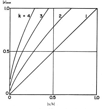
FIGURE 9. Effect of k on  $|\rho|_{max}$  for  $\lambda h$  equal to Infinity
